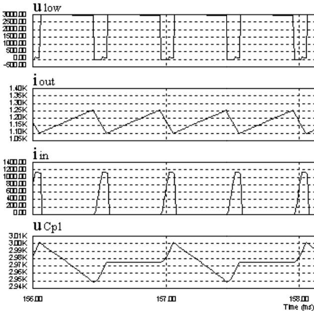
Fig. 3. Converter voltages and currents at drive mode
