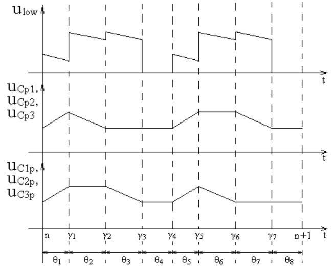
Fig. 5. Converter output voltage and voltages across capacitors in the drive mode
