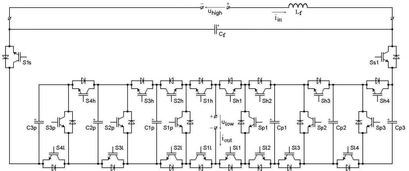
Fig. 2. Bidirectional six-stage dc-dc converter for an advanced DC electric locomotive
