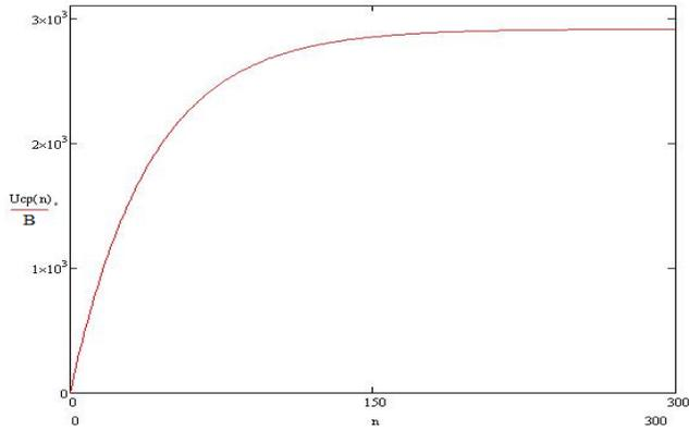
Fig. 6. The theoretical time dependence of the voltage across the capacitor
