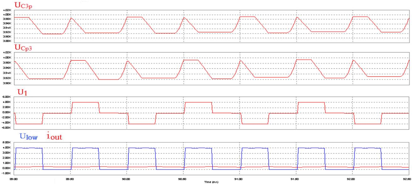
Fig. 9. Voltages across the capacitors, voltage of the primary winding of the transformer and output voltage and current of the bidirectional six-stage dc-dc converter with galvanic separation of the load
