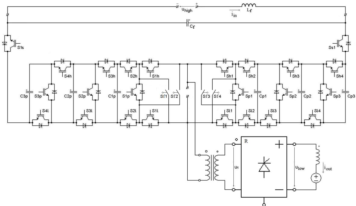
Fig. 8. Bidirectional six-stage dc-dc converter with galvanic separation of the load
