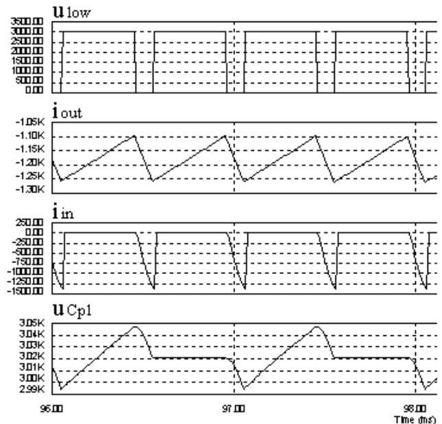
Fig. 4. Converter voltages and current at recuperation
