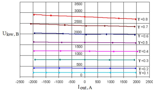
Fig. 7. The two-quadrant load characteristics of the converter
