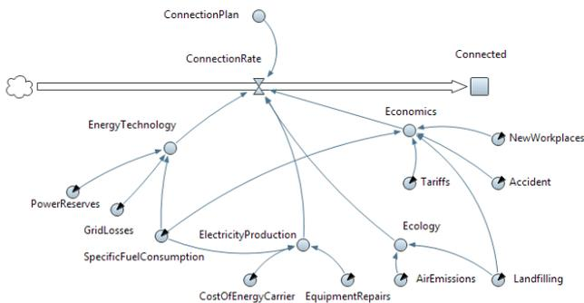
Fig. 6. The model of System Dynamics of introducing innovative technology of demand side management into the energy supply system.
