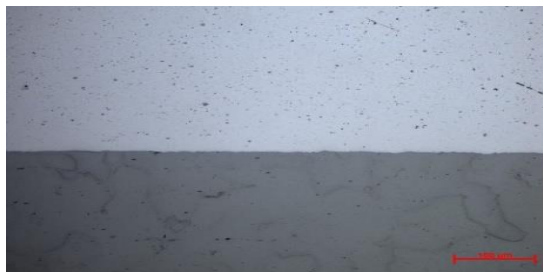
Figure 3 – The boundary of the welded joint
